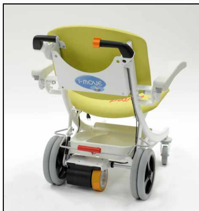
Motorized wheel including battery
