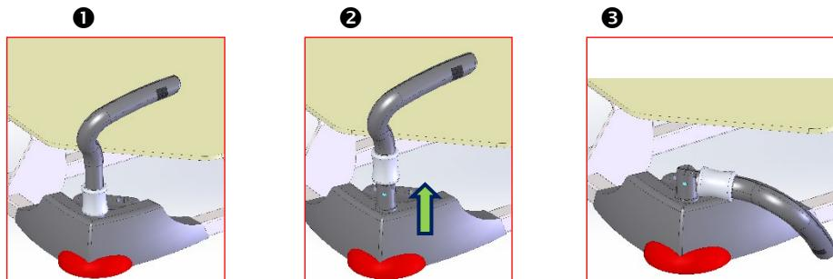
In order to reposition the handles, lift them and replace the ring in its low position. Check that they are positioned correctly.
