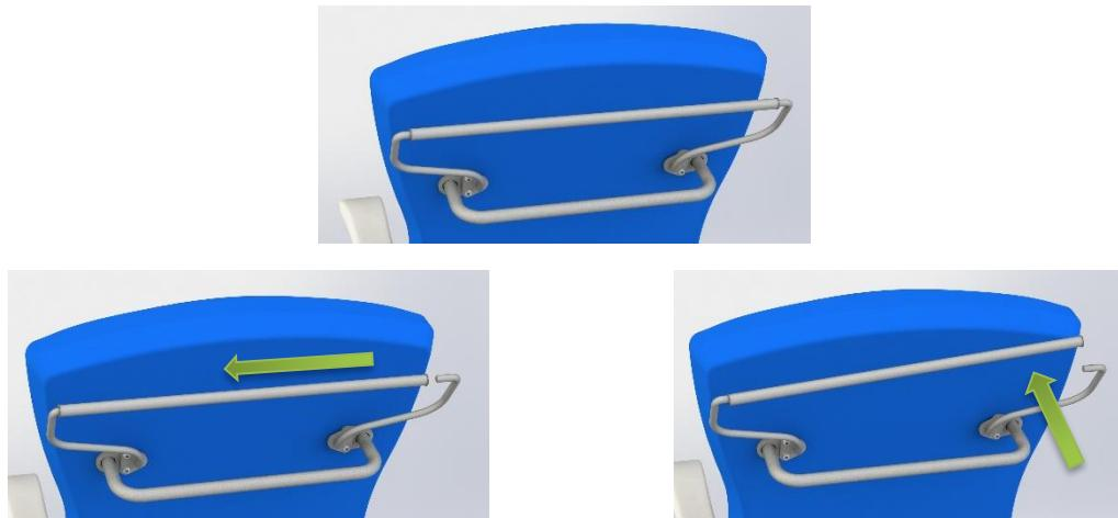
Pull the tube to the left and raise it slightly to slide the paper roll on, then pull the tube to the left once more to reposition it in its housing.
