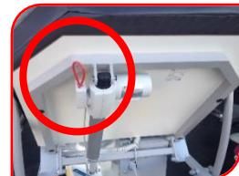
**If the emergency manual unlock has been used, lower the backrest with the remote control to its lowest position to reset operation. See [2.5.3.2 BACKREST POSITION RESET](#).**
